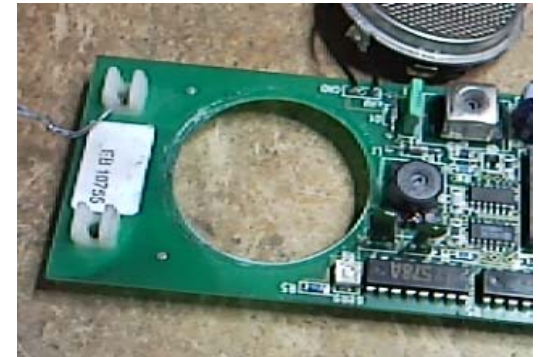
Figure 1. Use the knife to carefully dislodge the glue around the ultrasonic element.
