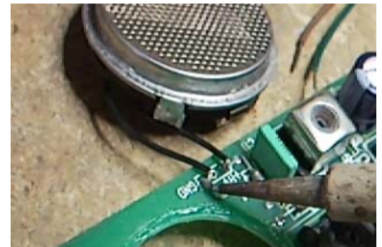
Figure 2. Using a soldering iron, pull the leads marked GND and HV.
