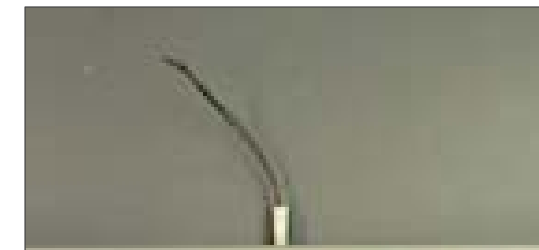
Figure 3. The "pigtail" can be detached from the rest of the kit via the white connector, making it easier to solder to the existing rangecard.
