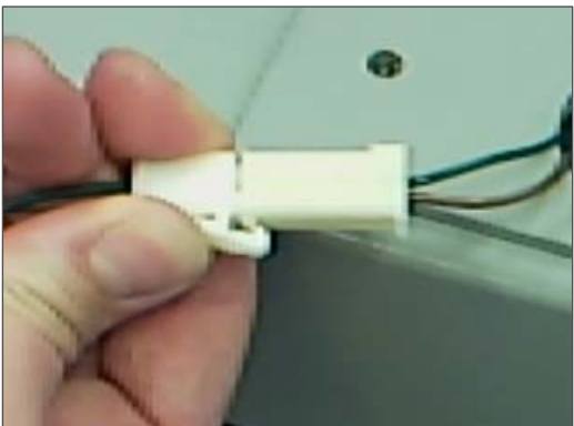
Figure 4. Ensure that the connector is in place properly by listening for the click.
