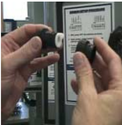
4. Loosen and remove the bayonet locking nut.
